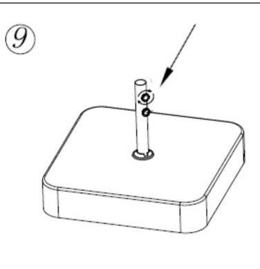
Fastern the 2 locking bolts in position to finish assembly.
