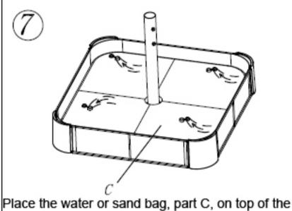
non-woven sheet and fill with water through the 4 holes. Each section must be filled separately and plugged with cap. We recommend using funnel to fill bag. Also can fill with sand instead of water.
