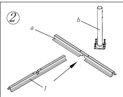
Create an X shaped base with the new rail, Part I, and Parts a and b originally sold with the offset umbrella.
