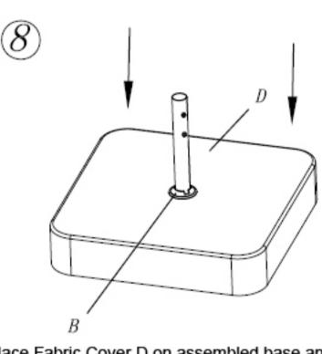
Place Fabric Cover D on assembled base and add the Trim Ring B to the post.
