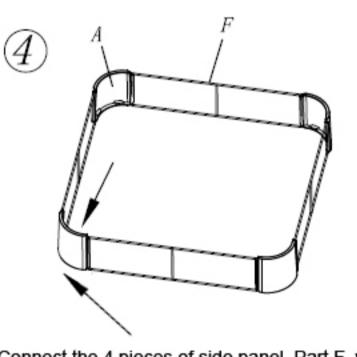
Connect the 4 pieces of side panel, Part F, with the 4 pieces of corner blocks, Part A. Pieces should snap together.
