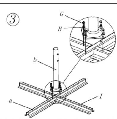
Add the base support tube, Part b, to the X base with 4 pieces of bolt G and 4 pieces of washer H.
